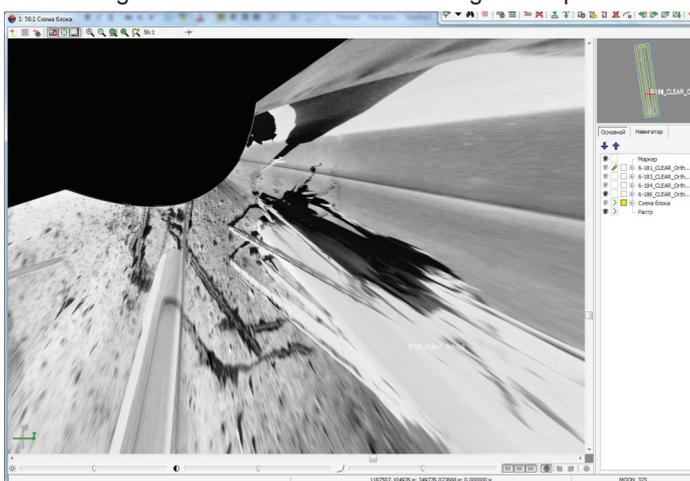
fig. C. Example of orthorectified panorama with a part of module Luna-17 and Lunokhod's track.
